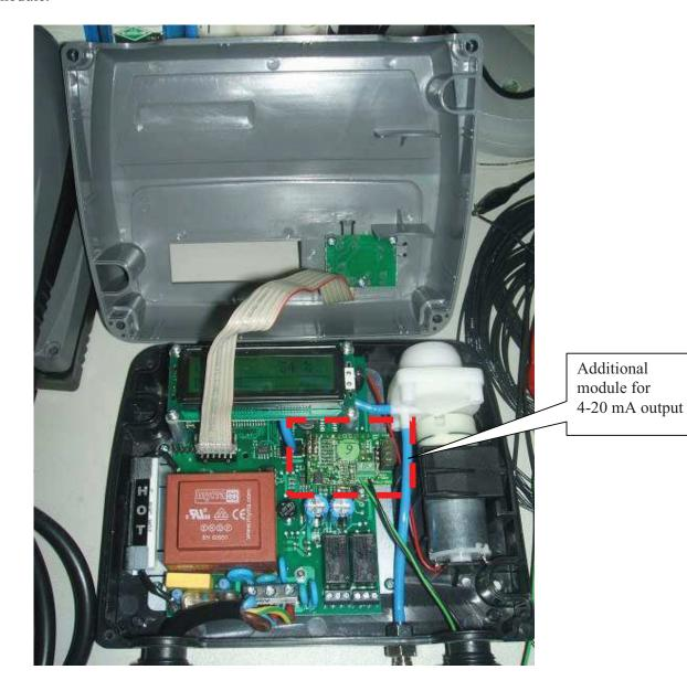
It is possibile to choose between active functioning mode (**self pwr**) and passive functioning mode (**loop pwr**) through the connector shown in the pictures.
